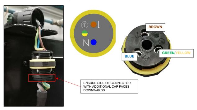
FIGURE 2, TERMINAL CONNECTIONS
